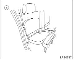
To access the jump seat extension ① on the passenger's side jump seat only pull up ② on the extension to unfold it to the open position. Then unfold the two support legs ③ and lower the jump seat to the full open ④ seating position.
