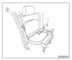
1. To access the jump seat extension (1) on the passenger's side jump seat pull up (2) on the extension to unfold it to the open position. Then unfold the two support legs (3) and lower the jump seat to the full open 4 seating position.
