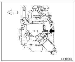
**QR25DE** engine **ENGINE SERIAL NUMBER**
