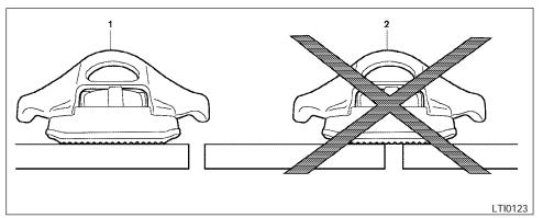
1 correct installation, 2 incorrect installation
