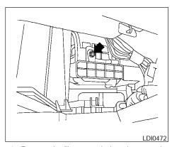
2. Remove the filter cover bolt and remove the filter cover.
