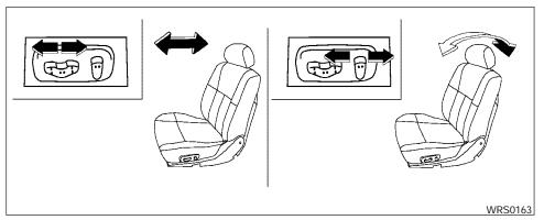
The reclining feature allows adjustment of the seatback for occupants of different sizes for added comfort and to help obtain proper seat belt fit (see "Precautions on seat belt usage" later in this section). Also, the seatback can be reclined to allow occupants to rest when the vehicle is stopped.
