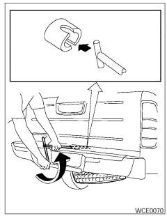
Seat the T-shaped end of the jack rod into the T-shaped opening of the spare tire winch. Apply pressure to keep the jack rod engaged in the spare tire winch and turn the jack rod counterclockwise to lower the spare tire.  Once the spare tire is completely lowered, reach under the vehicle, remove the retainer chain, and carefully slide the tire from under the rear of the vehicle.
